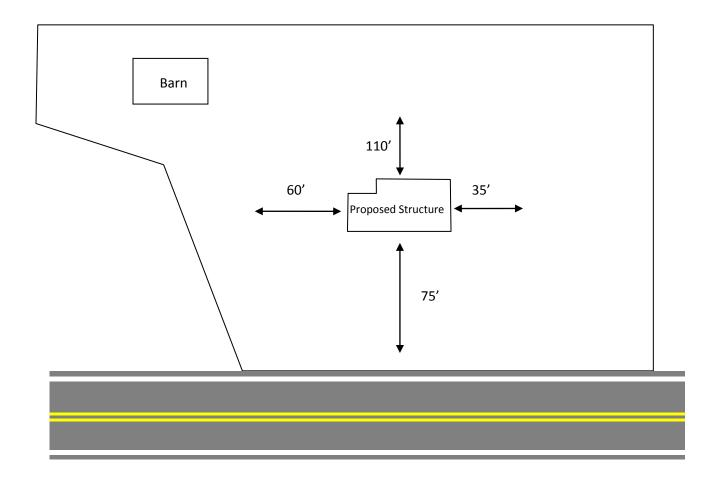
The Site Plan should show all structures that are on the property and the distance from the property lines to the proposed structure.
